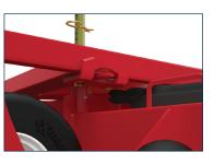
**CONVENIENT DECK LATCH** Changing the height of cut has been made easy with the added deck latch. Rather than holding the deck while changing the height of cut, the deck will now lock into place making it easier on operators.
