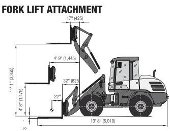
Operating load over total lift range: 4,188 lbs (1,900 kg) Operating load in transport position: 6,834 lbs (3,100 kg)\* "With rear axie weights
