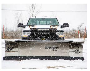
bottom channel • Nine reinforcing 1/4 in. laser-cut steel ribs • 1/2 in. cutting edge with integrated curb guards
