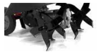
Tilling Depth up to 11"
